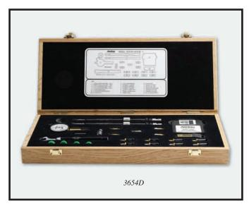
The Anritsu Calibration Kits contain all the precision components and tools required to calibrate your VNA or VNMS for 12-term error-corrected measurements in the connector style of your choice. Components are included for calibrating male and female test ports as required. The kits support calibration with opens, shorts, and broadband loads. Option 1 adds sliding terminations and a pin depth gauge where required.
